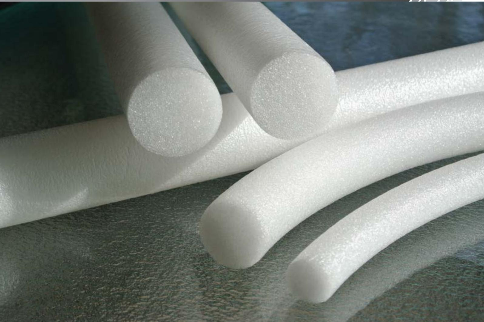
EASY-FORM™ Closed Cell Backer Rod is a compressible, closed cell polyolefin foam tube with an outer skin. It is used as a backing for cold applied sealants in expansion/construction joints and building seal applications.
